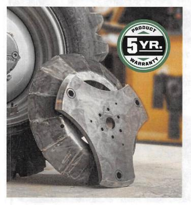
Diamond's proprietary Tri-Hex mulching disc on our rotary mowers provides greater inertia in tough conditions, and prevents material build-up between the deck and blade carrier. The disc is constructed of 1" thick 50,000 psi rated steel with hardened, replaceable inserts, giving you unparalleled durability and easy blade maintenance.
